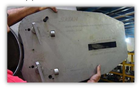
Whole the ink unit is easily dischargeable from the machine by only 3 screws. There is an electric crane on the machine for helping the operator put the ink unit down to the ground or mount on the machine.
